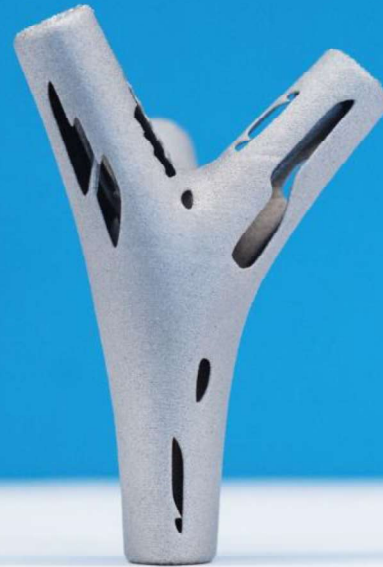
N-AM 10 - Topology optimized Steel Node.
