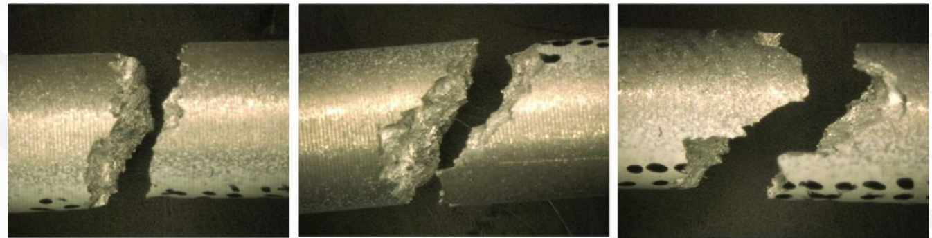
Tensile specimens and breaking pattern of AlSi10Mg
