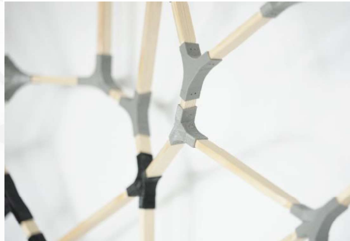
Zoom-In of the 1:20 model. The model is made of wooden sticks and 3D-printed FDM plastic nodes.
