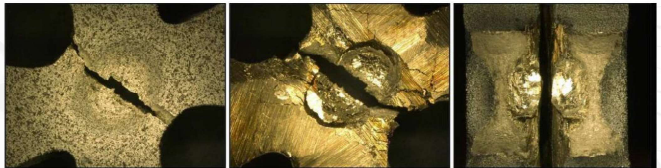
Validation Tests of X-form specimens made of Stainless-steel 316L
